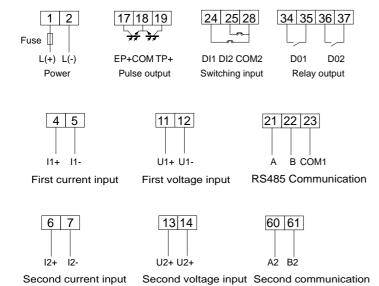
Note: The second DC input channel and DI and DO functions are optional.
