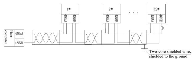
It is recommended to add a matching resistor between A and B of the end meter, and the resistance range is 120  $\Omega$  -10 K  $\Omega$  .
